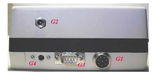
*Fig. 3.* Back panel of MEB-2c: G1 – probe input; G2 – charger input 1; G3 – RS232 output; G4 - charger input 2.
