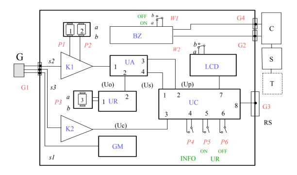
**Fig. 1.** Block diagram of MEB-2c: G -probe; K1- amplifier of Barkhausen voltage; K2 – amplifier and analyzer of reference signal; BZ – internal supplier; UA - Barkhausen signal analyzer; UR – threshold voltage source; UC – microprocessor unit; GM - current generator; LCD - screen; W1 – power switch; W2 – back light switch; ; P1, P2- gain switches; P3 - threshold voltage switch; P4 – INFO switch; P5 – UR ON switch; P6 – UR OFF switch; C – charger, S - power pack, T - transformer;
