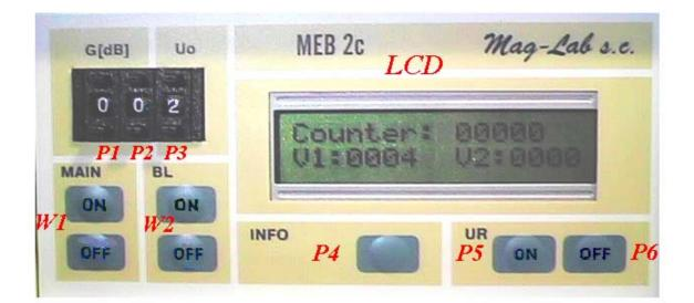
**Fig. 2.** Front panel of MEB-2c: W1 – power switch (MAIN); W2 – back light switch (BL); LCD - screen; P4 – switch INFO; P5 – switch UR ON; P6 - switch UR OFF; P1, P2 – gain switches G [dB]); P3 – threshold voltage switch.
