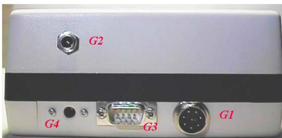
**Fig. 3. Back panel of MEB-2c:** *G1* – probe input; *G2* – charger input 1; *G3* – RS232 output; *G4* - charger input 2.
